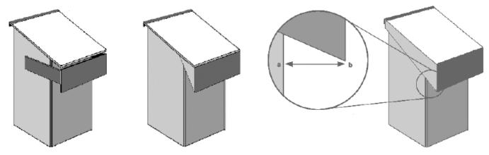
The distance of the baffle from the front of the box (a to b in the diagram above) should be at least equal to the diameter of the entry hole. As the possum needs to climb under the baffle, the clearance has to be big enough to let him through.
